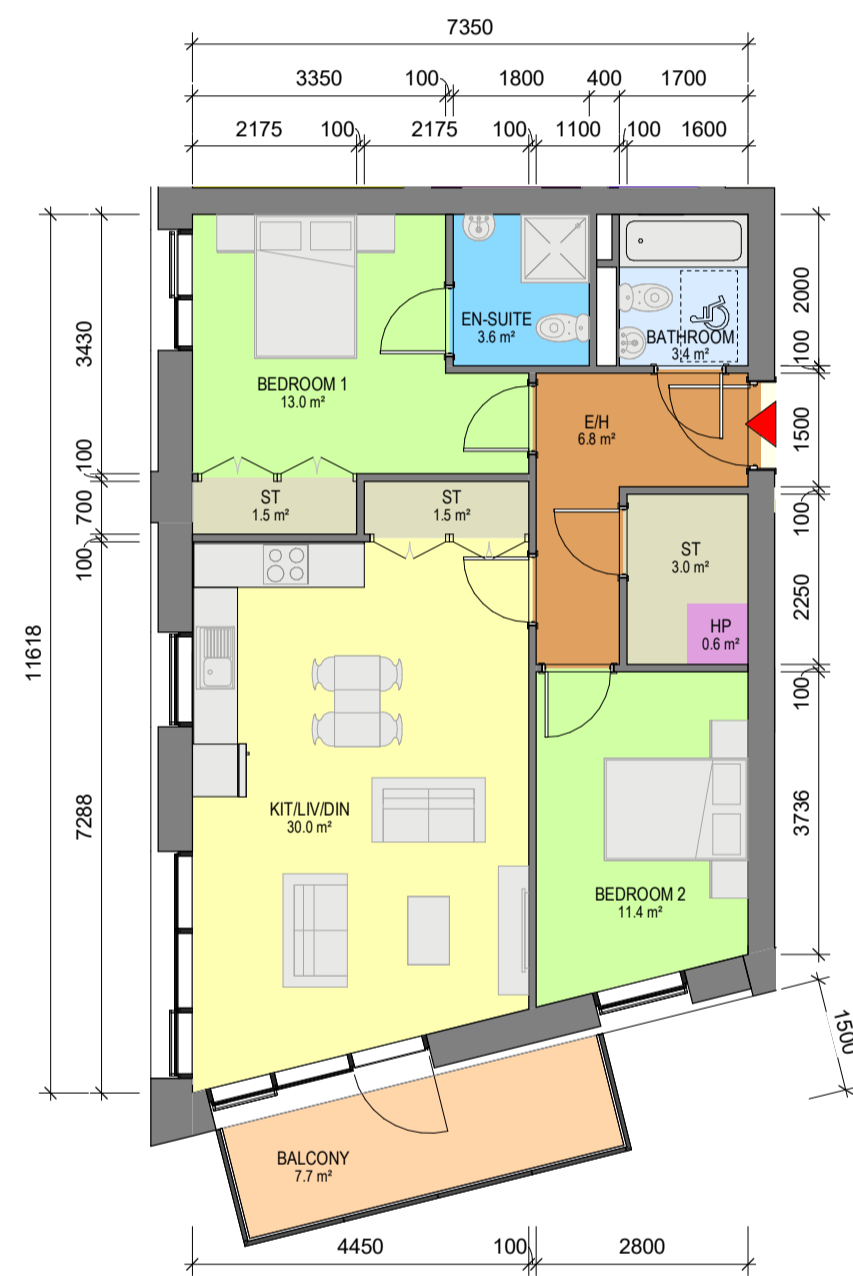
6 Apartment Type 2BB 1 : 100 - 2 BED, 4 PERSON APARTMENT - NET INTERNAL AREA (NIA) Areas shown in plan - GROSS INTERNAL AREA (GIA) : 78.66sqm
