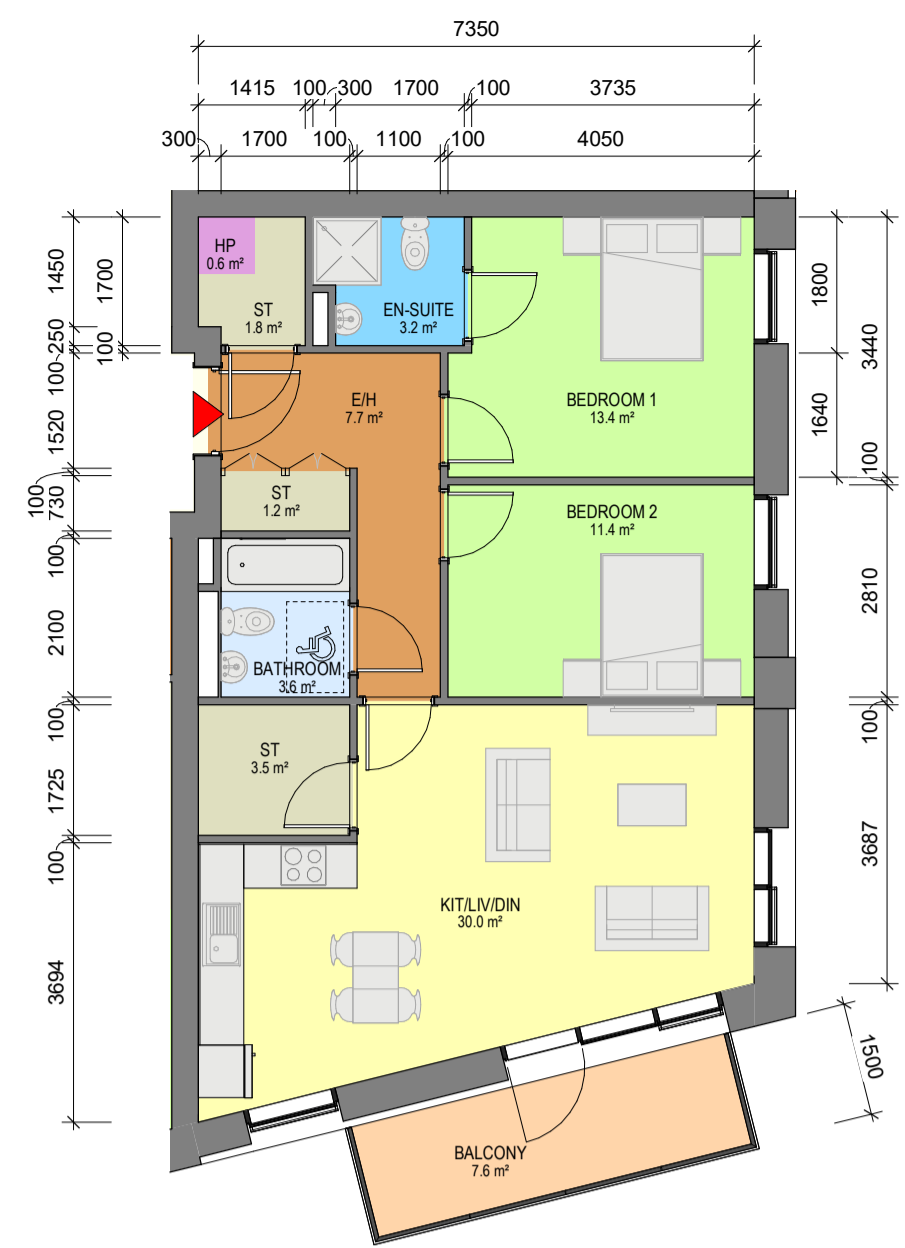
2 Apartment Type 2AX 1 : 100 - 2 BED, 4 PERSON APARTMENT - NET INTERNAL AREA (NIA) Areas shown in plan - GROSS INTERNAL AREA (GIA) : 80.40sqm
