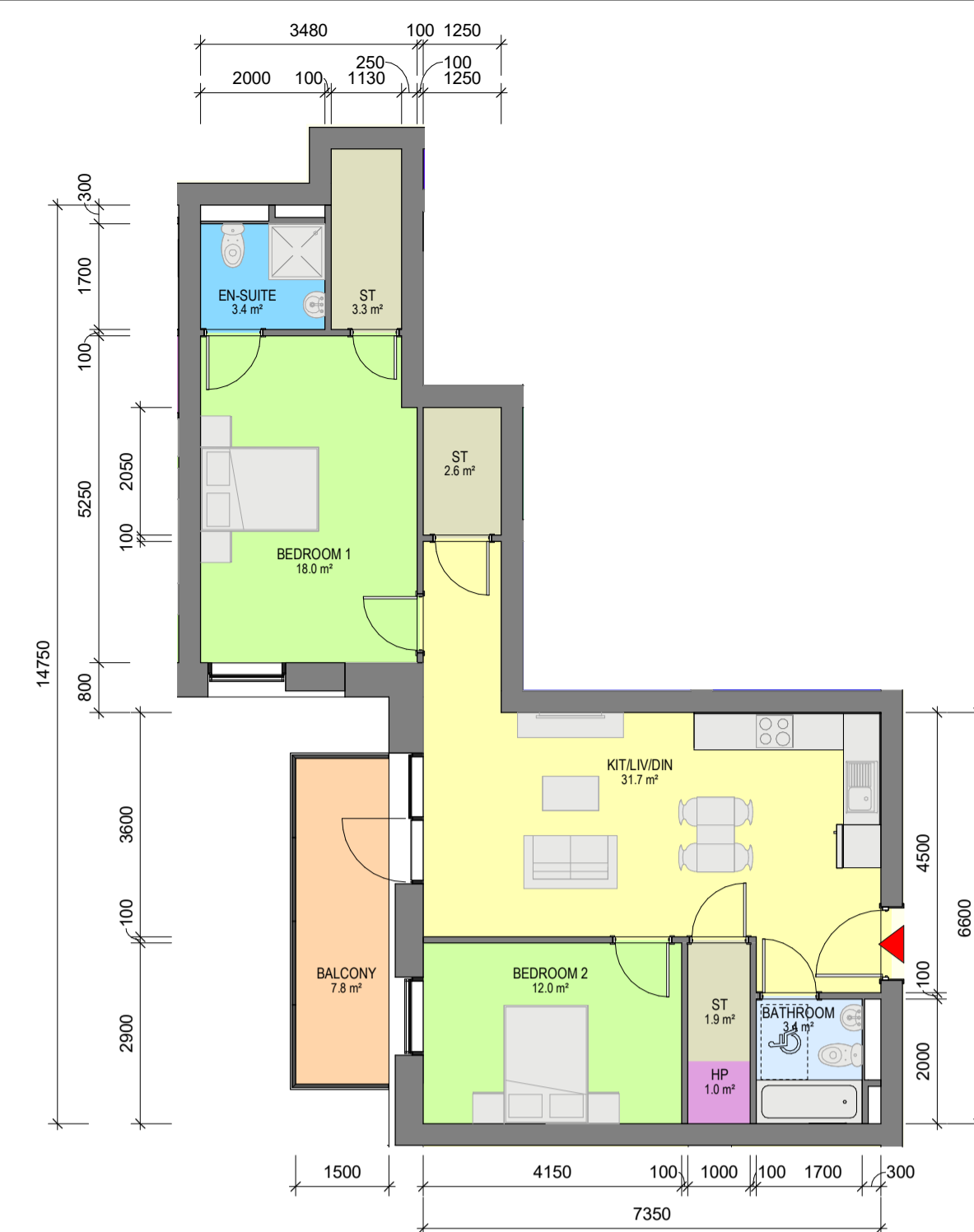
4 Apartment Type 2AZ 1 : 100 - 2 BED, 4 PERSON APARTMENT - NET INTERNAL AREA (NIA) Areas shown in plan - GROSS INTERNAL AREA (GIA) : 80.83sqm
