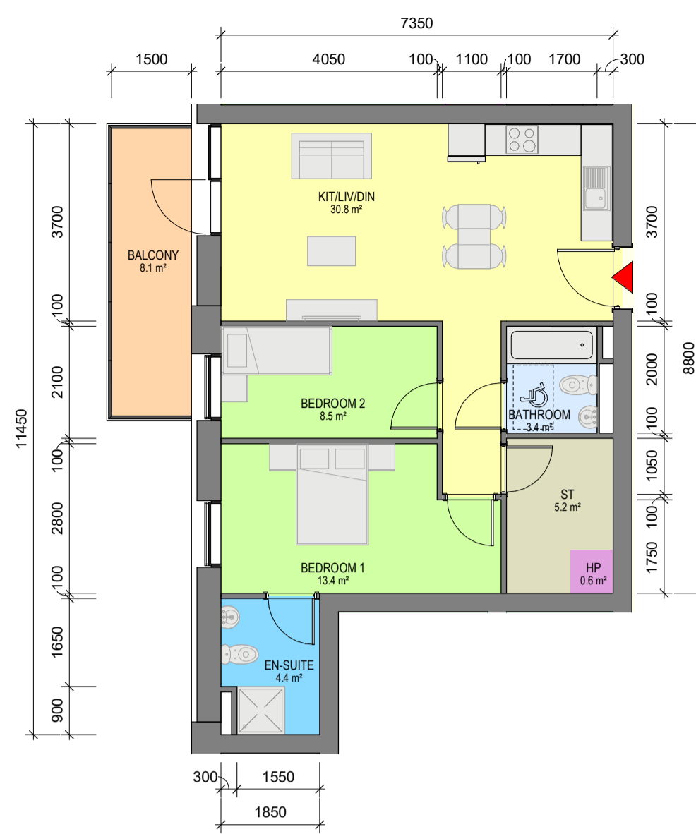
3 Apartment Type 2AY 1 : 100 - 2 BED, 3 PERSON APARTMENT - NET INTERNAL AREA (NIA) Areas shown in plan - GROSS INTERNAL AREA (GIA) : 69.58sqm
